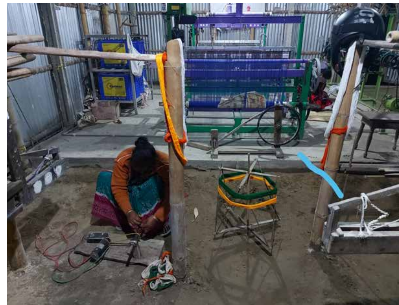
IMAGE 9: An installed solar powered loom bobbin drive in Nalbari, Assam
