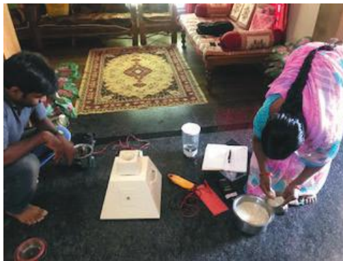
Grinding idli batter with DC mixer grinder
