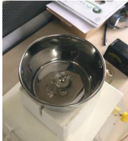
Prototype of DC mixer grinder during lab testing
