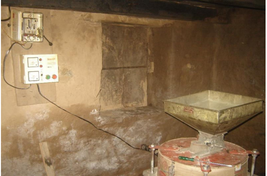
Photo 6.9: Atta Chakki in Topania based on Hydropower from Karmi III
