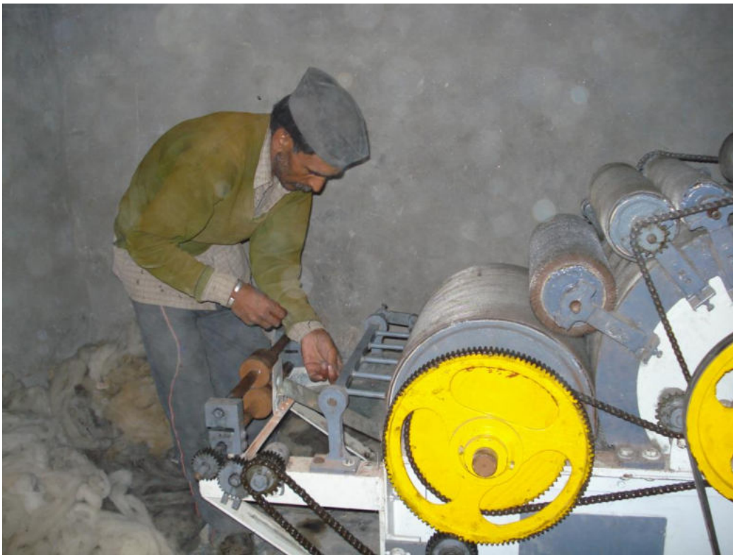
Photo 7.4: Wool Carding Machine in Agunda
