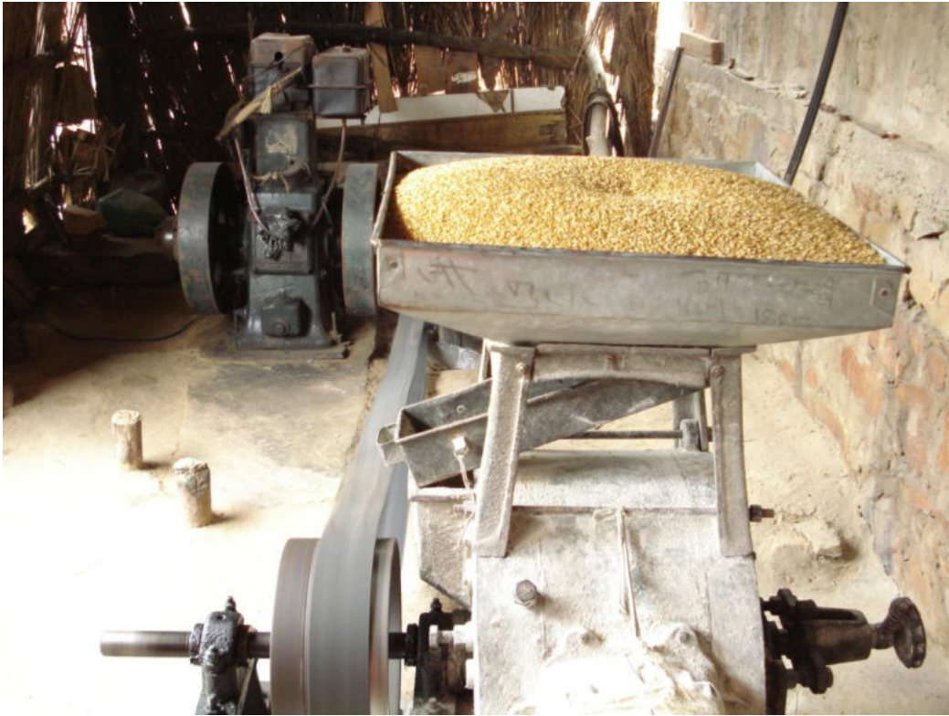
Photo 2.15: Atta Chakki using motive power from the Gasifier, Nagla Ramoli
