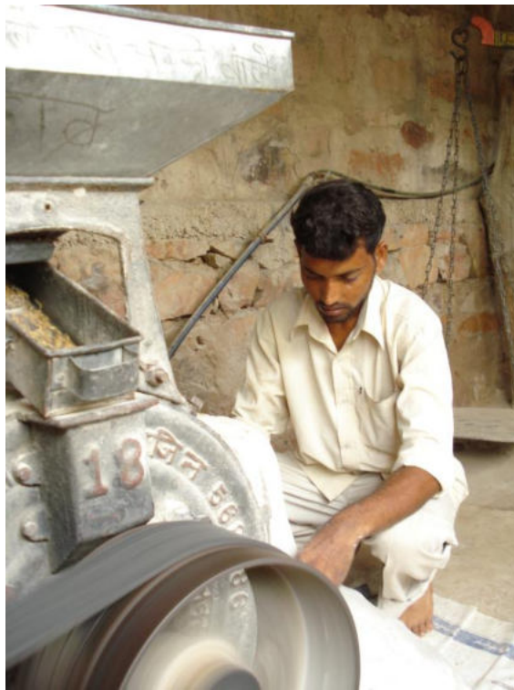
Photo 2.16: Atta Chakki converting Wheat into Flour at Nagla Ramoli
