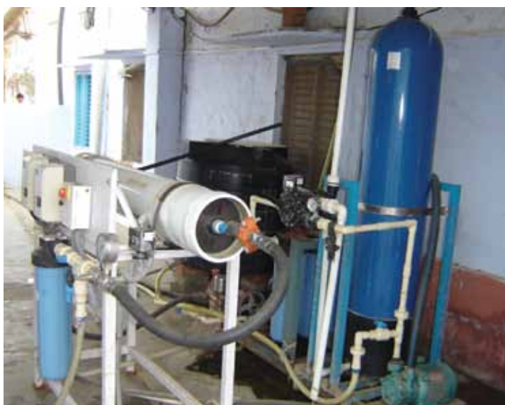
Figure 4: Barefoot College's solar RO desalination unit, Kotri, Rajasthan 26 Source: (Barefoot College) 27
