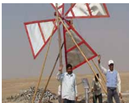
Figure 17: Bamboo prototype of the low-cost windmill (left) and modified model installed for salt farming. Source: (NIF) 109
