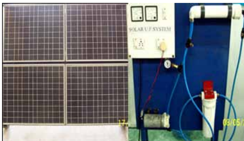
Figure 9: BARC solar powered water purifier based on ultrafiltration
