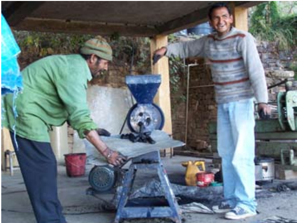
Making fuel briquettes with residual charcoal
