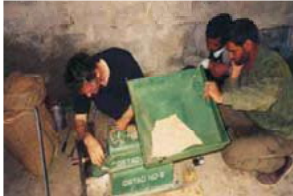
Rice huller being set up
