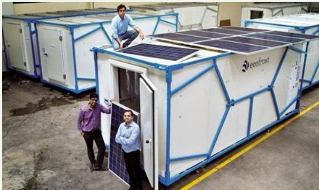
Ecofrost: a solar cold storage
