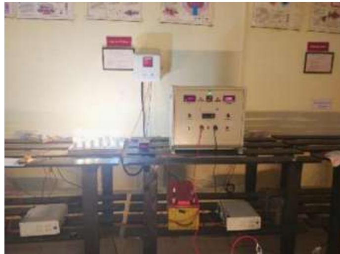
Figure 2 Discharging of a lead acid battery carried out at constant current at CES lab at PCCOE (source: CES)
