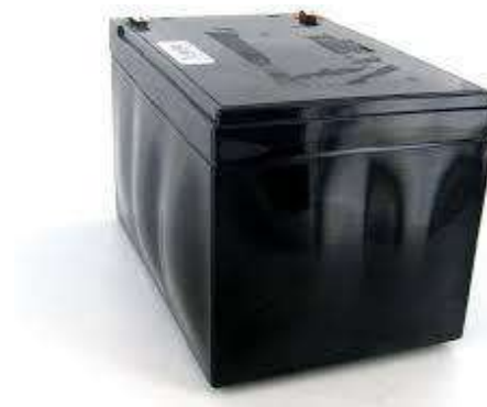
Figure 56 Image of a bulged lead acid battery
