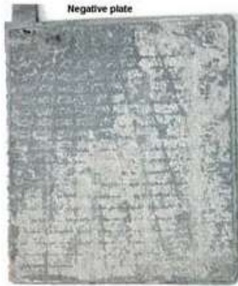
Figure 14 A hard sulfated negative plate
